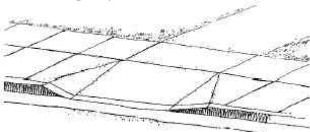
*Figure 4-35: Jogging the sidewalk back from the street provides a level landing for pedestrians on narrow sidewalks.*
